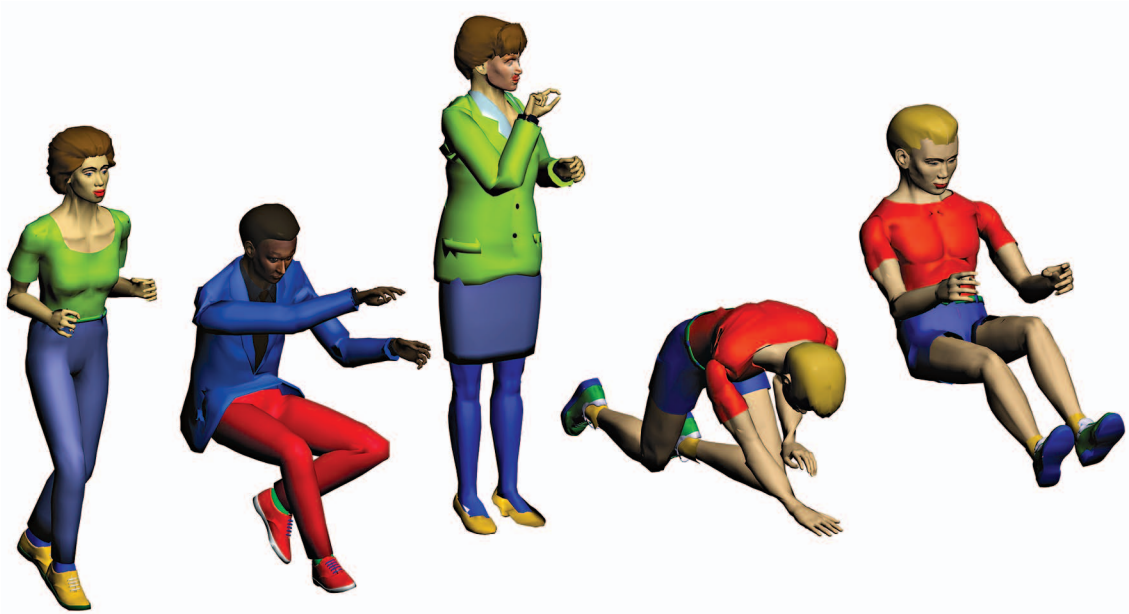
Figure 2. Digital human models in various predefined postures, with clothes generated in ErgoMAX. ErgoMAX offers predefined postures in seven categories: bagger (putting things into bags), bending, kneeling, lying, sitting, standing, and walking.
